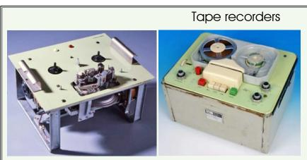
Jesenik tape recorder (left) and Hostyn playback machine (right. The reel to reel tape in a cassette allowed rapid change and vertical positioning of a stack of recording machines.
