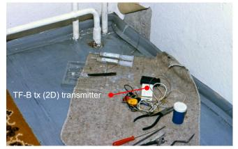
TF-B (2D) system: Preparation and installation of a microphone through a small hole in the wall to the adjacent (to be intercepted) apartment known as Operational Object. Note the TF-B tx transmitter (2D) unit and a (black) battery which were placed in a neighbouring apartment. The transmission to the TF-B rx receiver in the Operational Support Point (right photo) was via central heating pipe and neutral mains, providing both units were in the same group.
