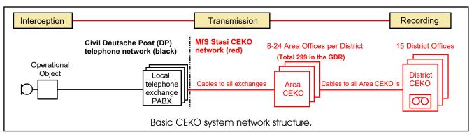
The District CEKO in a MfS Stasi District Office was connected by cables to all the MfS Area offices where the (usually unmanned) Area CEKO system with distribution frames connecting to Deutsche Post telephone exchanges and other distribution facilities, for example leased Post Office
