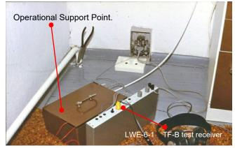
Connecting a LWE-6-1 TF-B test receiver to an AC mains power point in a Operational Support Point located at the top apartment of the same block as the Operational Object. The Operational Support Point was fitted in a metal cassette (behind the test receiver) comprising a 31140 TF-B rx receiver and a 31121 TF-tx transmitter, the latter connected to a telephone subscriber line. From this point the intercepted audio was routed to the CEKO system.
