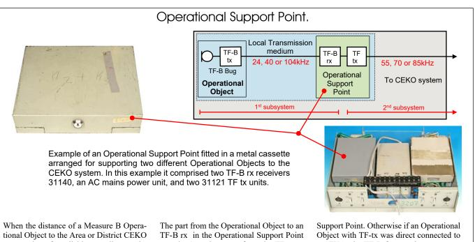
was too long for reliable recording, or the use of Measure B 2 A (AC mains based) or B 2 C (doorbell cable based), an Operational Support Point (German = Operative Stützpunkt) was installed. This was principally a form of repeater. Depending on the situation, an Operational Support Point could be located in in any suitable but trusted location and exceptionally in a telephone exchange (installed in a separate locked room).
